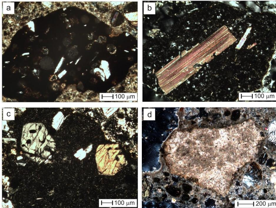
Fig. 2. Microphotographs of samples at optical microscope in polarized light. a) Pozzolanic fragment with crystals of plagioclase immersed in a glassy groundmass with vesicles texture. b) Pozzolanic fragment with macrocrystals of biotite. c) Pozzolanic fragment with macrocrystals of clinopyroxene. d) Example of calcite nodule present in the samples, occurring naturally in Vesuvian ash [4].
