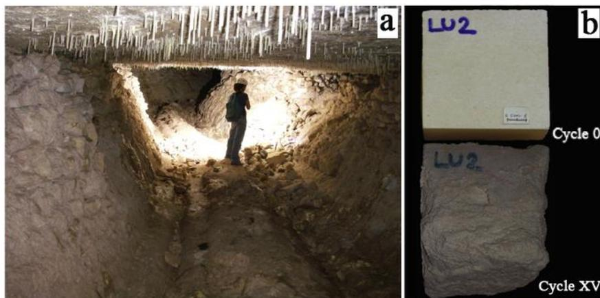
Fig. 1. a) Historic underground quarry “latomia” of the “*calcare a lumachella*” (Maddalena peninsula - Syracuse); b) specimens of “*calcare a lumachella*” before and after the salt crystallization tests.
