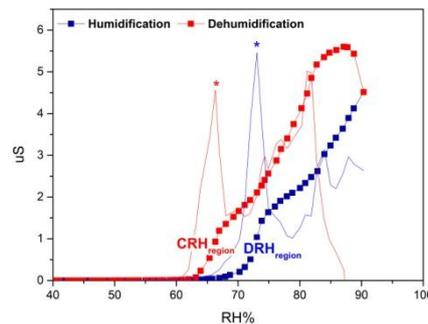
Fig.1: Typical conductance Vs RH curve obtained for PM<sub>2.5</sub> sample.
