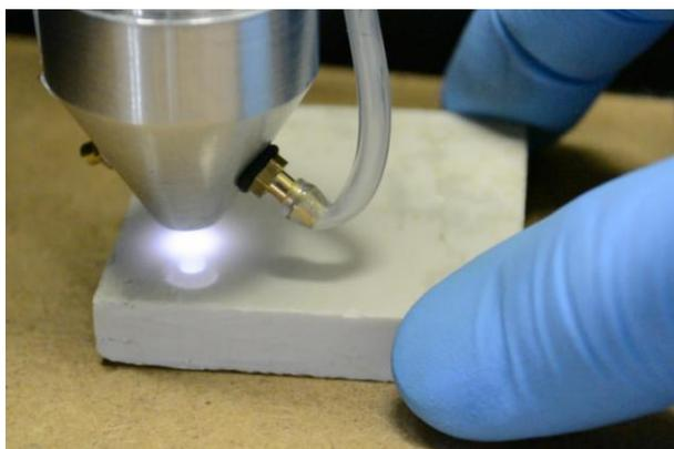
Fig. 2: Plasma removal of the self-diagnostic coating on
