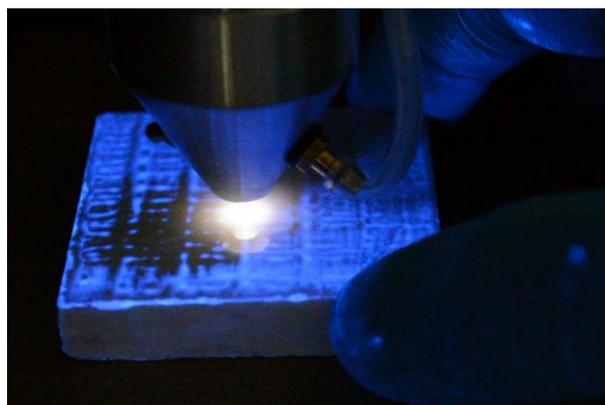
Fig. 3: Plasma removal of the self-diagnostic coating on
