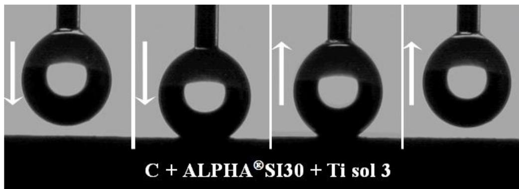
Color and static contact angle measurements were carried out for hydrophobic and superhydrophobic systems before and after 10h of UV exposure (Table 1). The treated samples did not show both a visible colour and contact angle variations even after UV irradiation (always  $\Delta E^* \leq 4$ ,  $\Delta \theta^* \leq 3$ ).
