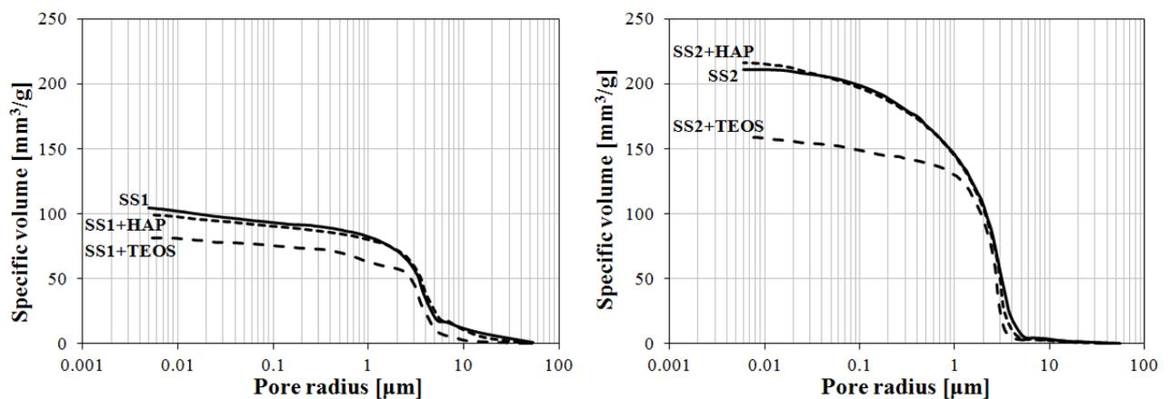
Fig. 1. Pore size distribution of untreated and treated samples
