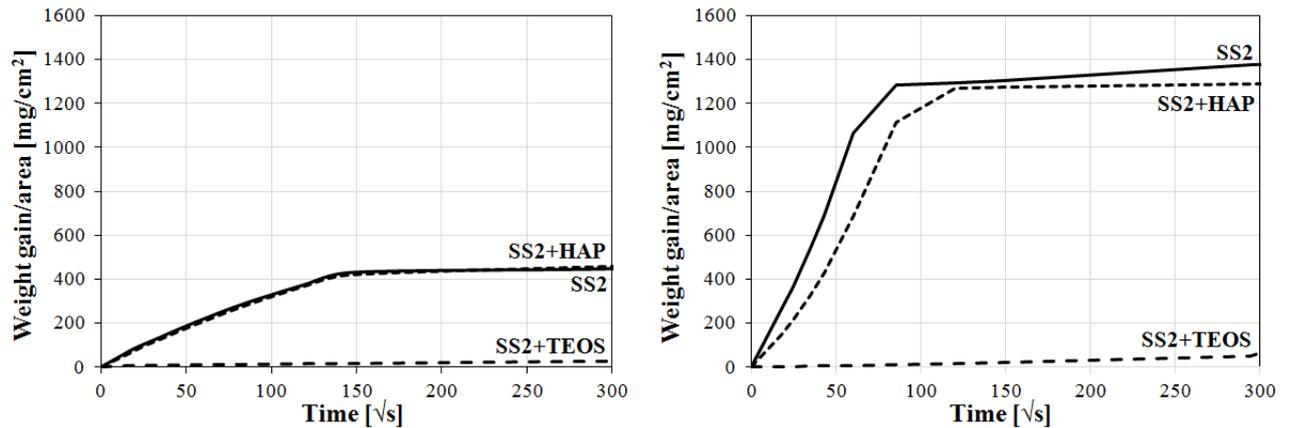
Fig. 2. Water sorptivity of untreated and treated samples
