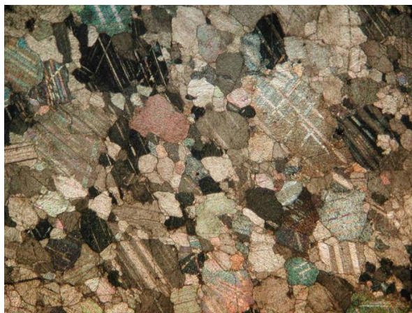
Figure 3 – Photomicrograph of Paros marble from a white tessera. Transmitted light, crossed nicols. Horizontal field of view is 5,2 mm.
