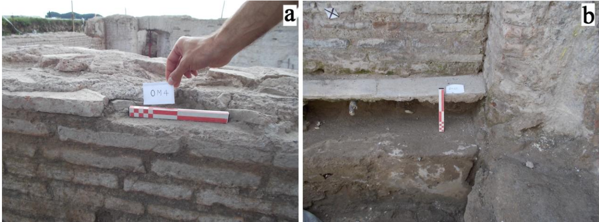
Fig. 1. Two examples of sampled mortars: a) bedding mortar; b) paving mortar.
