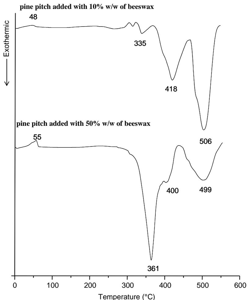
Fig. 1. DSC analysis of pine pitch added with different percentage of beeswax.
